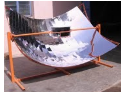
Concentrating solar collector
